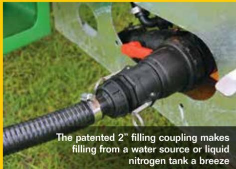
The patented 2" filling coupling makes filling from a water source or liquid nitrogen tank a breeze
